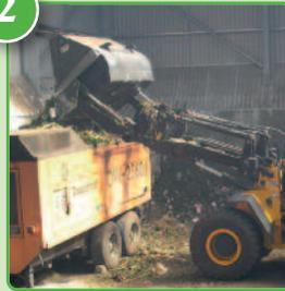
A load that passes the inspection is shredded and broken down into smaller pieces that will compost more quickly.
