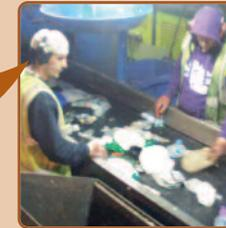
Cartons are removed by hand then baled and sent for recycling. The plastic and foil components are used for a variety of new items and the cardboard is used in the corrugated bits of new cardboard.
