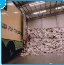
Paper is recycled in the UK. The paper is unloaded and sent to drum pulpers that act like giant washing machines. Large, unwanted items are rejected here. The material is now known as 'stock'.
