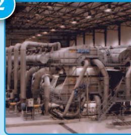
The stock enters centrifugal cleaners (like spin dryers) that remove smaller contamination like staples and grit. Ink is removed by pumping air into the water; the ink sticks to the bubbles which rise to the top forming a scum on the surface that is floated off. Any remaining glues are removed when hydrogen peroxide is added and the temperature raised.
