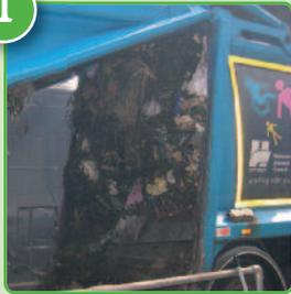
The vehicle arrives at the composting facility where the contents is weighed and tipped into a reception building. The load is inspected and if there is too much contamination it may be rejected and sent to landfill.
