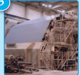
The stock is sprayed onto rollers and trapped between two belts of fabric to squeeze out some of the water - this forms a wet sheet of paper. It passes over sets of heated rollers to dry out.
